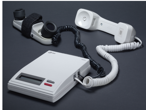
Figure 2: AT&T TSD-3600 Telephone Security Device (photo courtesy of the author)
